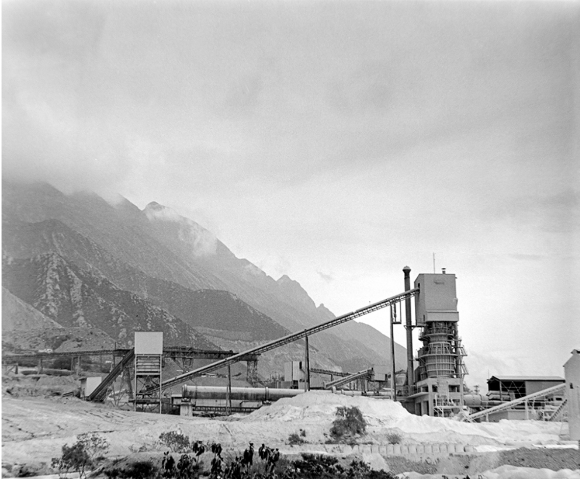
Figure 2: San Ángel stone quarry. It is still in operation at the western end of the Cerro de las Mitras. This photograph shows the limestone extraction device, the crushers and chutes to turn them into fine sand, 2020.
