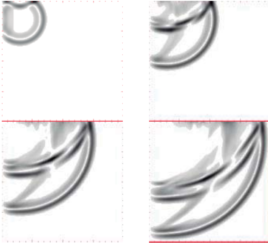
Figure 2: Snapshots for an elastic wave propagating through a homogeneous medium partitioned into four subdomains like a chess board. The size of the model is 2,000 \times 2,000 \text{ m}^2 and the snaps have been taken at a simulation time of 0.2, 0.4, 0.6 and 0.8 seconds.
