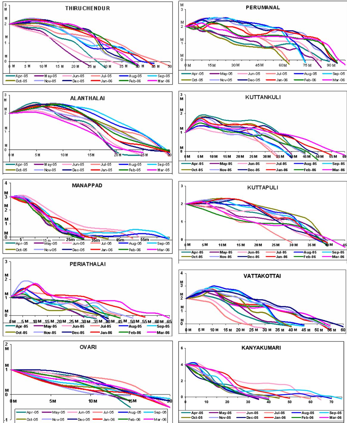
Fig. 7.- Monthly variation in beach profile along the study area. X-axis indicates distance from the reference point (m); Y-axis indicates elevation point (m).
