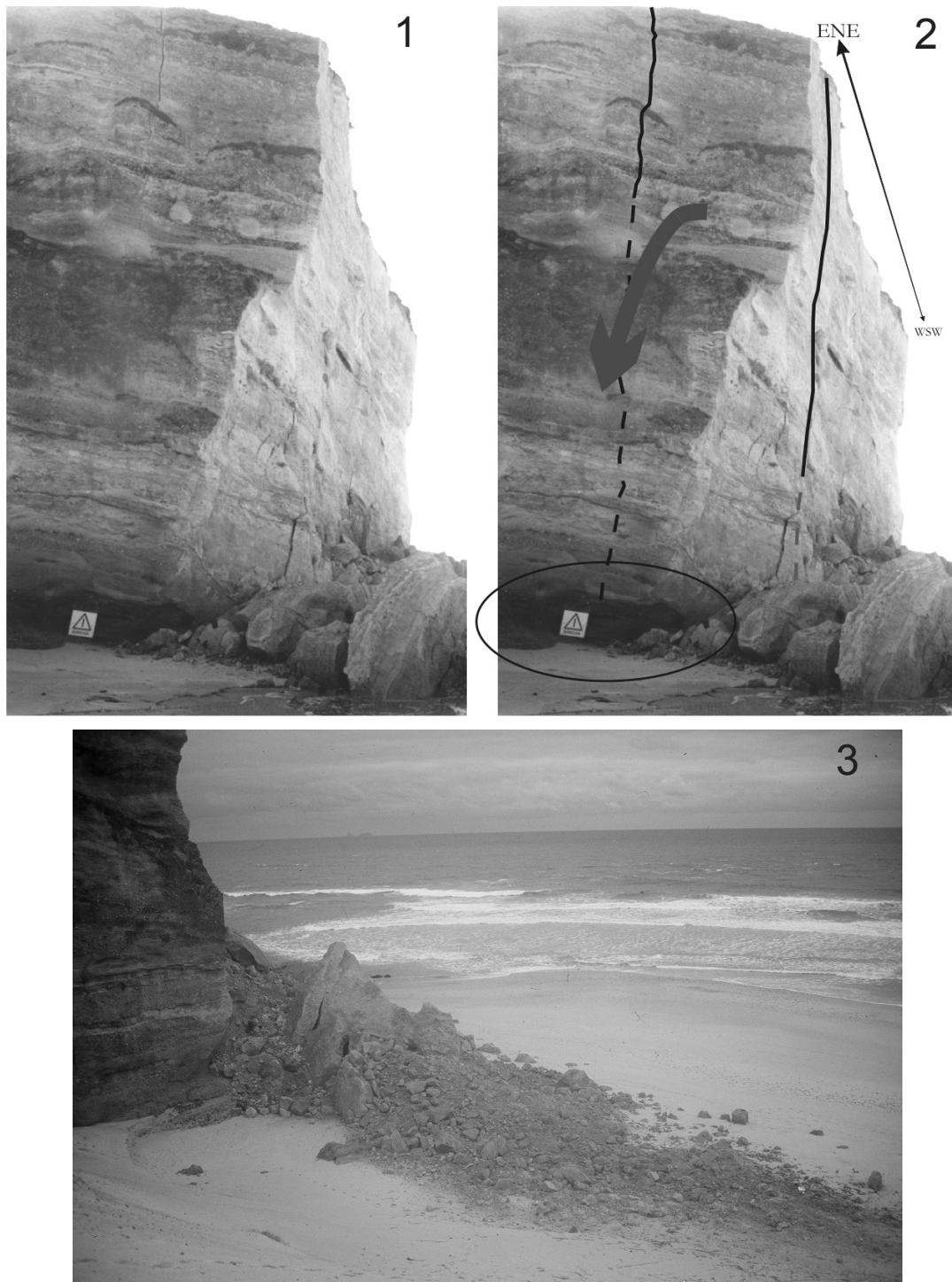
Fig. 7.- ENE sector of Gronho cliff affected by a topple at 14 December 1999. 1 and 2 - Full lines - main fractures; dotted line - probable fracture lines; ellipse - notch at the cliff base; the arrow points out the topple direction. 3 - Photo taken 4 days after the slope movements; the topple debris were dispersed to NE.
