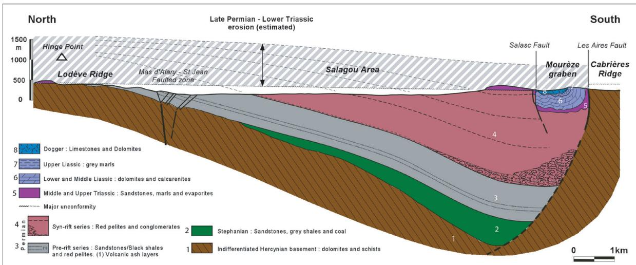
Fig. 2.- N-S-cross-section of the Lodève Permian basin; from Lopez and Petit (2003), modified.
