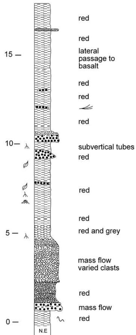
Fig. 17.- Stratigraphic section low in the higher red beds (Viar River section), where they are in lateral transition with upper basalt. Scale in metres.
