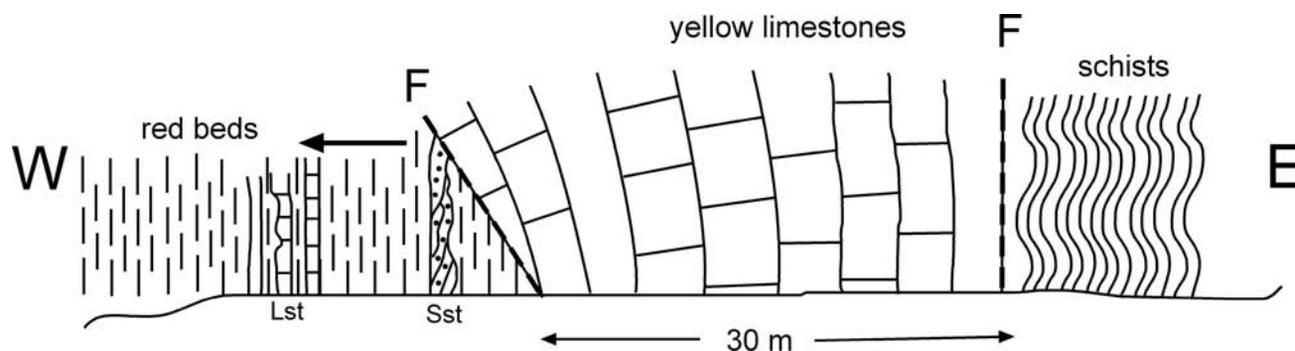
Fig. 30.- Section corresponding to an abandoned road cutting alongside the main road to El Pedroso. Red beds assumed to be Triassic are in thrust contact with presumed Mississippian cream coloured limestones. These, in turn, are in fault contact with Precambrian schists with bands of gneiss. This is the more important fault (see Fig. 2). Scale: 1:500
