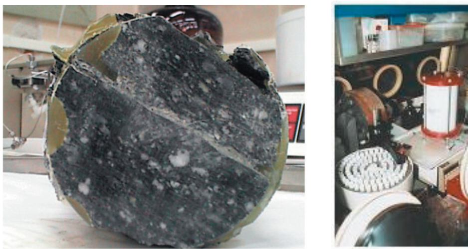
Fig. 2.- Example of a fractured core used for column transport experiments. The core came from the Grimsel Test Site.
