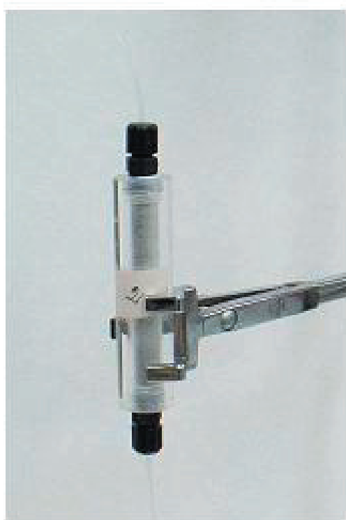
Fig. 6.- Small column for transport experiments with crushed crystalline rock.
