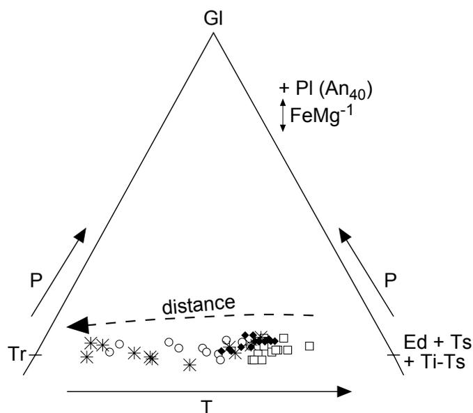
Fig. 8.- Qualitative thermobarometer (based on Castro *et al.*, 1996b) defined by a baricentric projection of amphiboles in the space Tr – GI – Ed + Ts + Ti-Ts, through the FeMg<sup>-1</sup> interchange and from PI (An<sub>40</sub>). The curve marks the compositional evolution (with respect to the distance to the Calabazares shear zone) of the Acebuches amphiboles (symbols as in figure 7).
