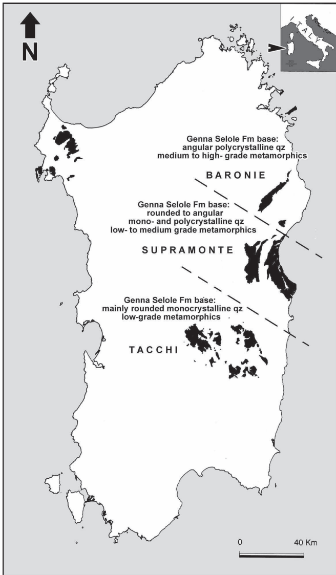
Fig. 16.- Composition of the Genna Selole Fm base in the diverse areas of Eastern Sardinia. Jurassic outcrops in black.
