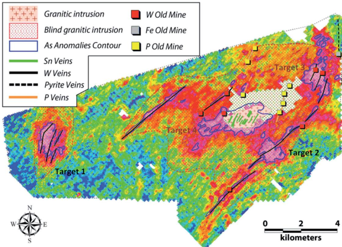
Fig. 2. – Map with schematic geological features of the Logrosan Project area and gradient plot of geochemical soil results for As on the background (modified from Mikhailov, 2014; E.N. Adaro, 1982).
