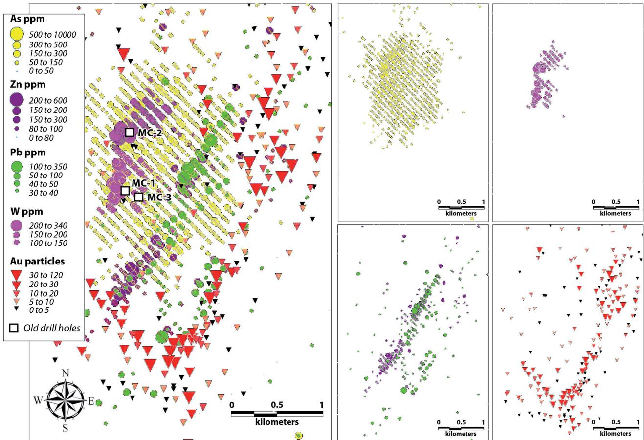
Fig. 3. – Geochemical map of the Target area 1 displaying soil sampling results for As, Zn, Pb, W; pan-concentrate sampling results for Au and old drill holes were made by MAYASA in 1980.
