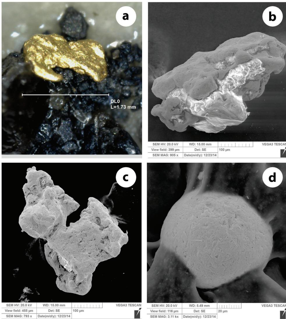
Fig. 6 – (a) Gold particle of 1.73 mm size. (b) BSE image of gold intergrowth with quartz (bright). (c) BSE image of gold particle with ore-crystalline morphology (d) BSE image of rounded gold grain with thin crater-like indentations and scratches in random directions (analyst Blinov I.).
