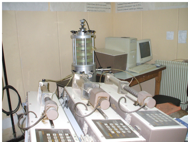
Fig. 4.- Photograph of the automated triaxial test setup.
