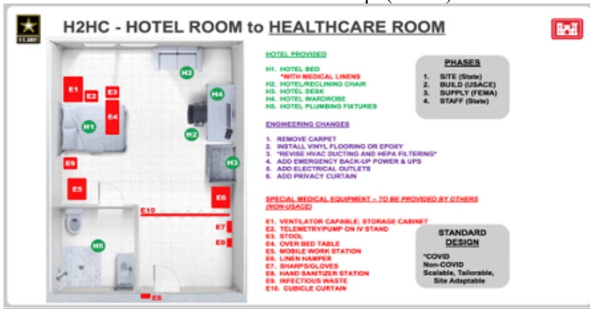
Figure 1. Plans to convert hotels into care rooms under the Hotel to Healthcare Concept (H2HC)
