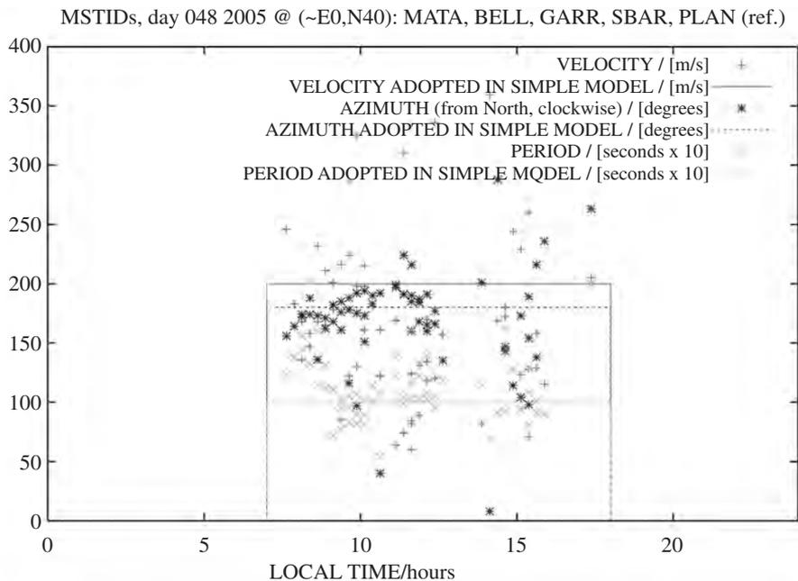
**Figure 9.-** Plot showing the compatibility of the actual and modeled MSTID characteristics (DMTID) during the experiment analyzed in this paper (day 048, 2005). The adopted values in the experiment, shown in Table 1, are also represented in the plot (velocity, azimuth and periods of 200 m/s, 180 deg and 1000 seconds, since 0700 to 1800 LT).
