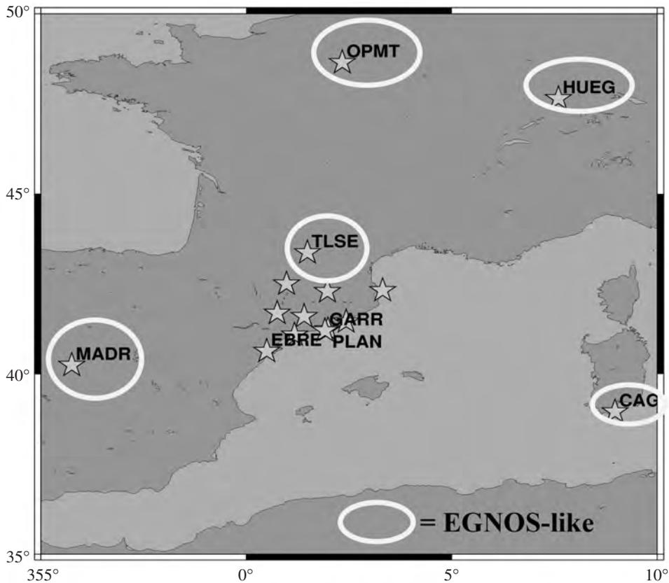
**Figure 7.-** Map indicating the reference receivers: encircled for large network and the remaining labelled ones for small network; the remaining receivers (non-labeled) are treated as roving users.
