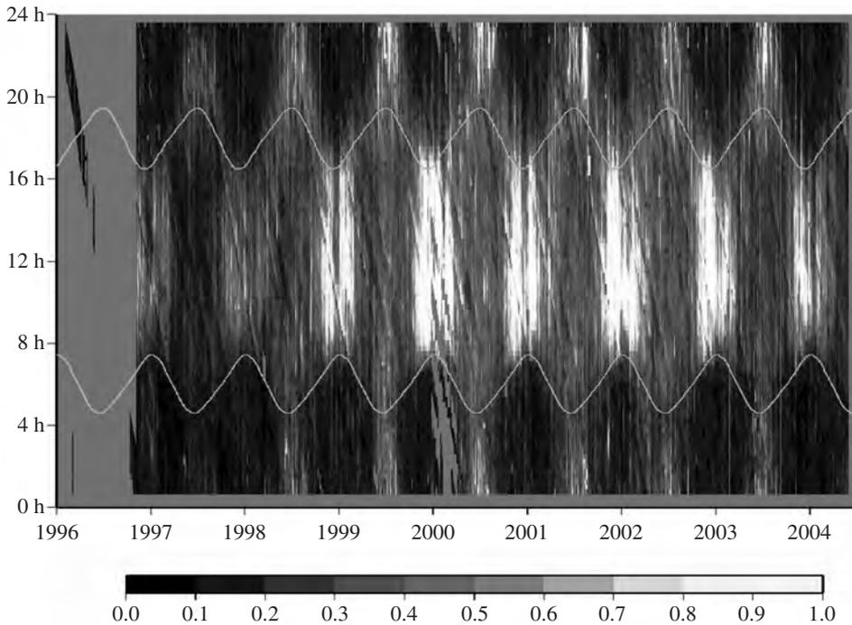
**Figure 5.-** Rescaled amplitude of MSTIDs detected over the EBRE GPS receiver (40.6N, 0.5E). Horizontal axis represents the day in years, and the vertical axis represents the local time in hours. The continuous line represents the Solar Terminator.
