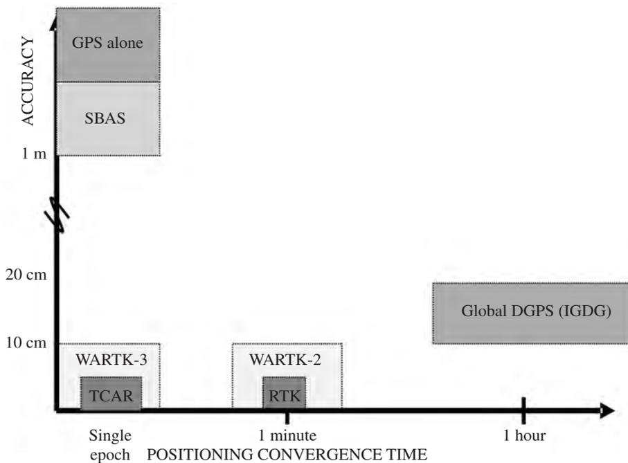
**Figure 2.-** Plot showing the accuracy versus positioning convergence time for different GPS systems. The WARTK system (WARTK-2 and WARTK-3) fills a gap, with sub-decimeter navigation errors at hundreds of kilometers baselines lengths. In the case of WARTK-3 such centimeter-level accuracy can be achieved instantaneously most part of the time.
