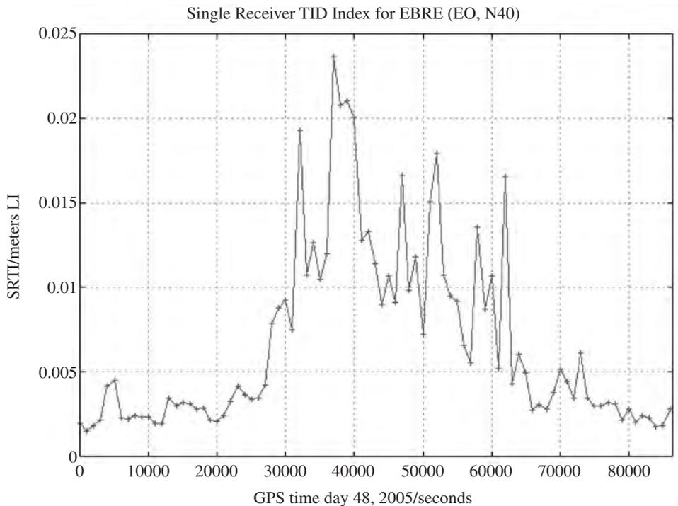
**Figure 8.-** Single Receiver TID Index computed for receiver EBRE, in terms of GPS time, for day 48 of 2005.
