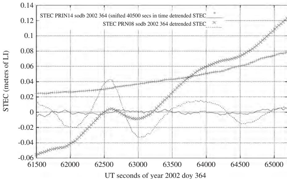
**Figure 4.-** Two examples of the detrending method acting over one STEC series without apparent TIDs (“x” and “-” signs, PRN14) and other where a TID is present (“+” sign and line, PRN08). In both cases the STEC has been divided by an obliquity factor in order to diminish the variation in the time window.
