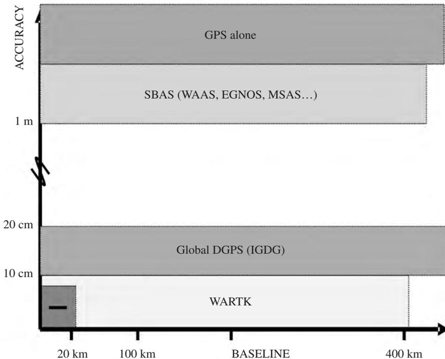
**Figure 1.-** Plot showing the accuracy versus baseline length (from the nearest reference site) for different GPS systems. The WARTK system (WARTK-2 and WARTK-3) fills a gap, with sub-decimeter errors at hundreds of kilometers' baselines. In the case of WARTK-3 such centimeter-level accuracy can be achieved instantaneously most part of the time (see next figure).
