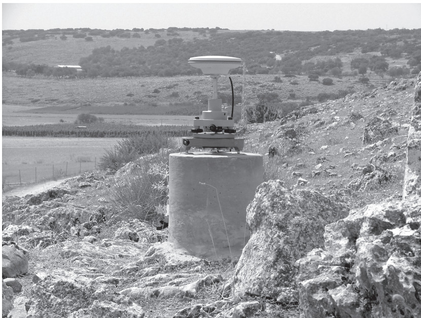
Figure 2. Reinforced concrete pillar anchored to rock in site 800.
