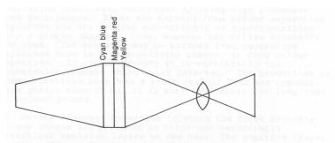
Schematic representation of a subtractive colour process
