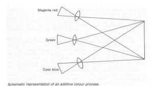
By way of three coloured light sources (blue, green and red) three black-and-white transparencies produced from the corresponding red, green and blue separations, are projected in superimposition.
