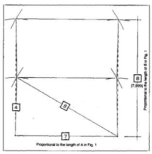
Fig. 2.—Geometrical construction of the ground-plan layout.
