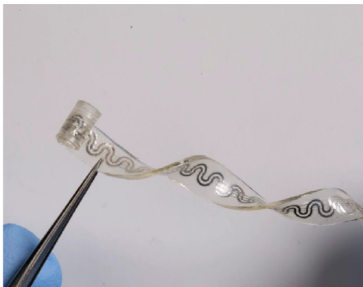
Researchers at Northwestern University created an implantable device that attaches to a nerve to deliver pain relief. Northwestern University
